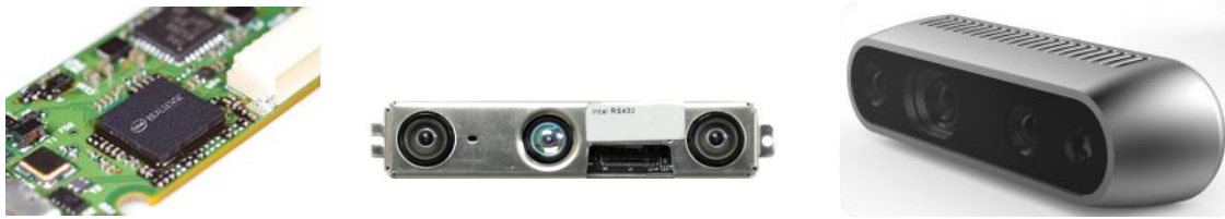
Fig. 7. Left: Intel RealSense™ D4m vision processor. Middle: Example of one of the Intel RealSense™ D4xx series depth modules encased in a steel case. RIGHT: Intel RealSense™ USB3 Depth Camera D435.
