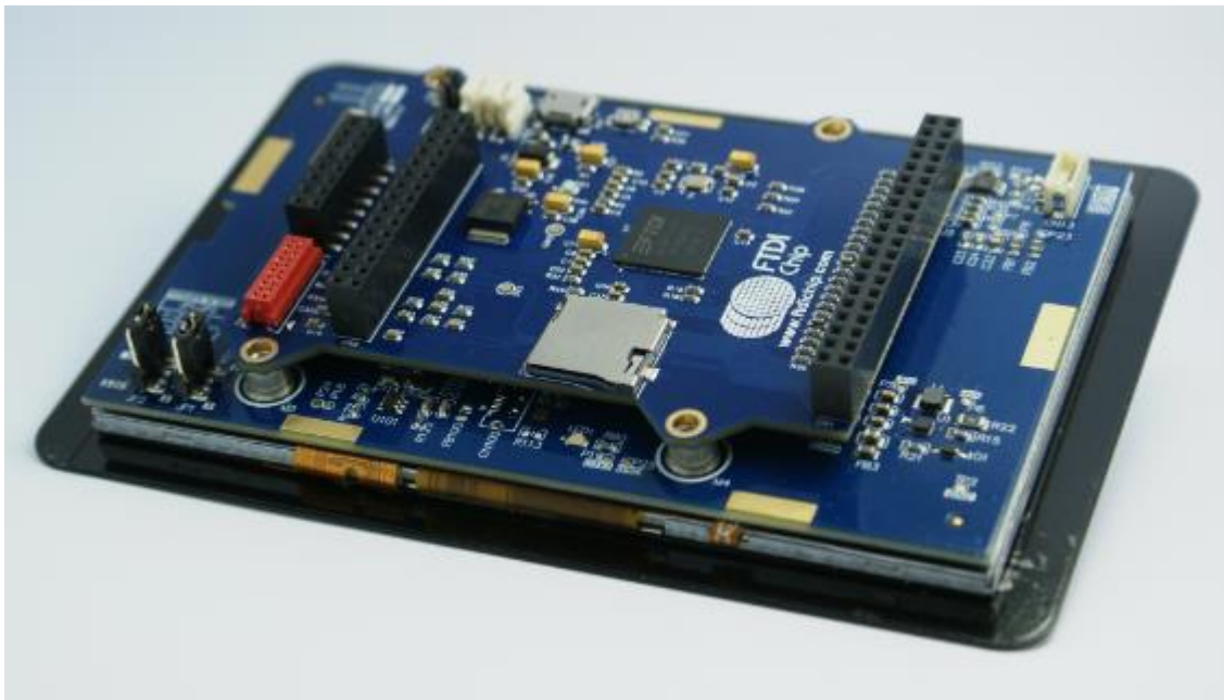
Figure 7-1 – ME813A-WH50C connects to MM900EV1A Module
