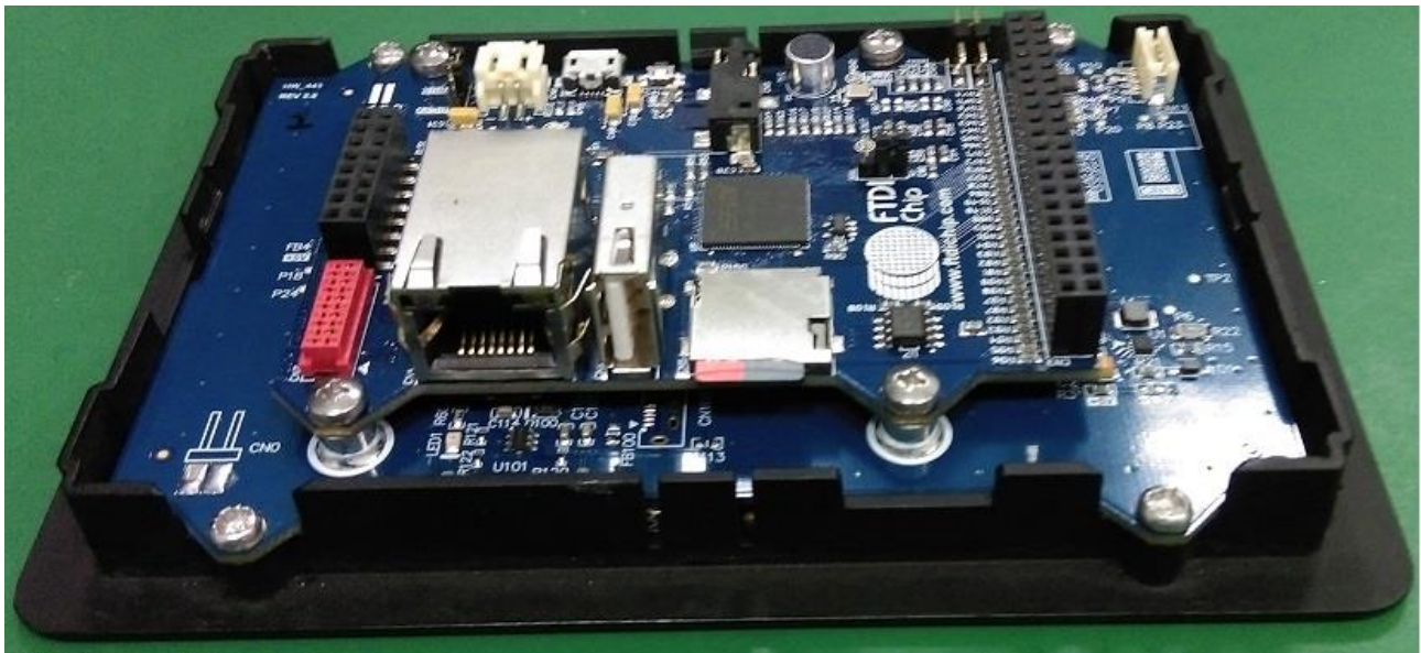
Figure 7-1 – ME812A-WH50R connects to MM900EV1A Module
