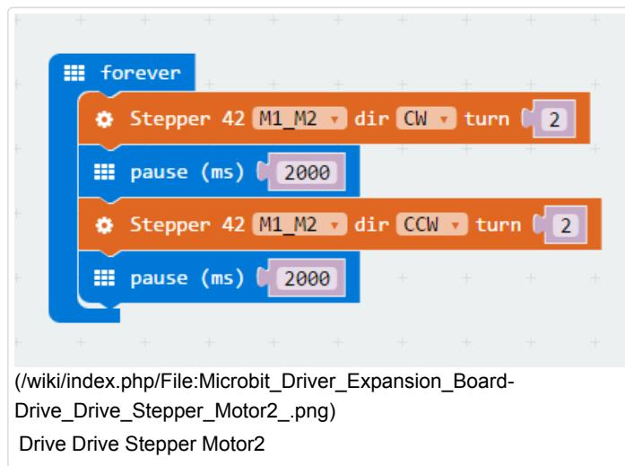
**Result:** When turned on, the stepper motor rotates clockwise for 2 turns, then rotates counterclockwise for 2 turns, in endless loop.
