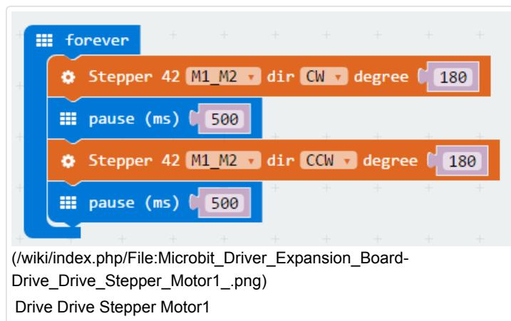
**Result:** When turned on, the stepper motor rotates clockwise 180°, then rotate counterclockwise 180°, in endless loop.
