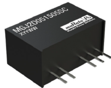
Figure 6. Typical 2 W IGBT driver DC-DC converter from Murata Power Solutions with 5.2 kV test isolation voltage, 3 pF coupling capacitance, optimised output voltages, zero minimum load requirement and safety agency ratings. The product is available with a selection of inputs and bipolar outputs to suit IGBTs and MOSFETs.
