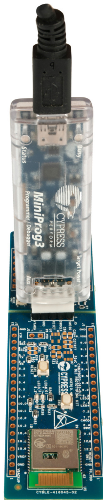
Figure A-15. Connecting the CY8CPROTO-063-BLE to a MiniProg3
