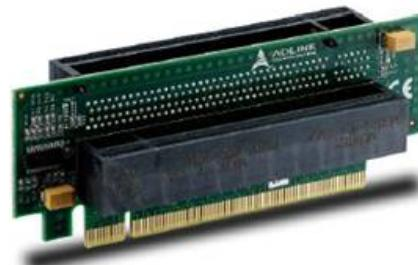
Insert the adapter card into the PCIe x16 slot of the Express-BASE7 carrier board as shown below.
