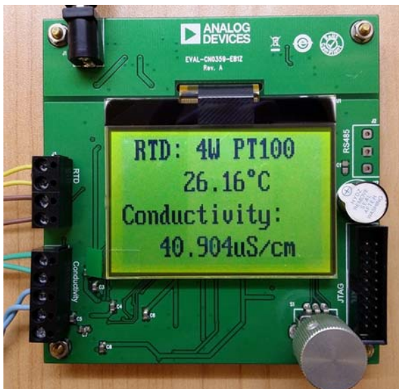
Figure 12. Photo of EVAL-CN0359-EB1Z Board Showing Home Screen in Measurement Mode
