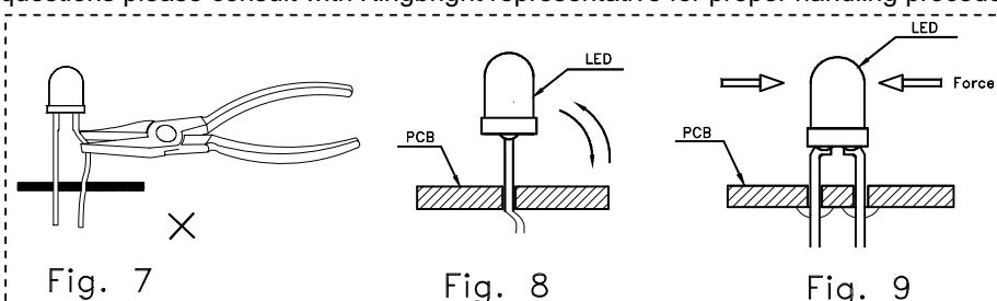
7. When bending the leads, the LED lamp should be secured by the upper part of the lead. Do not grip the epoxy lens during lead-forming bending the lead.
