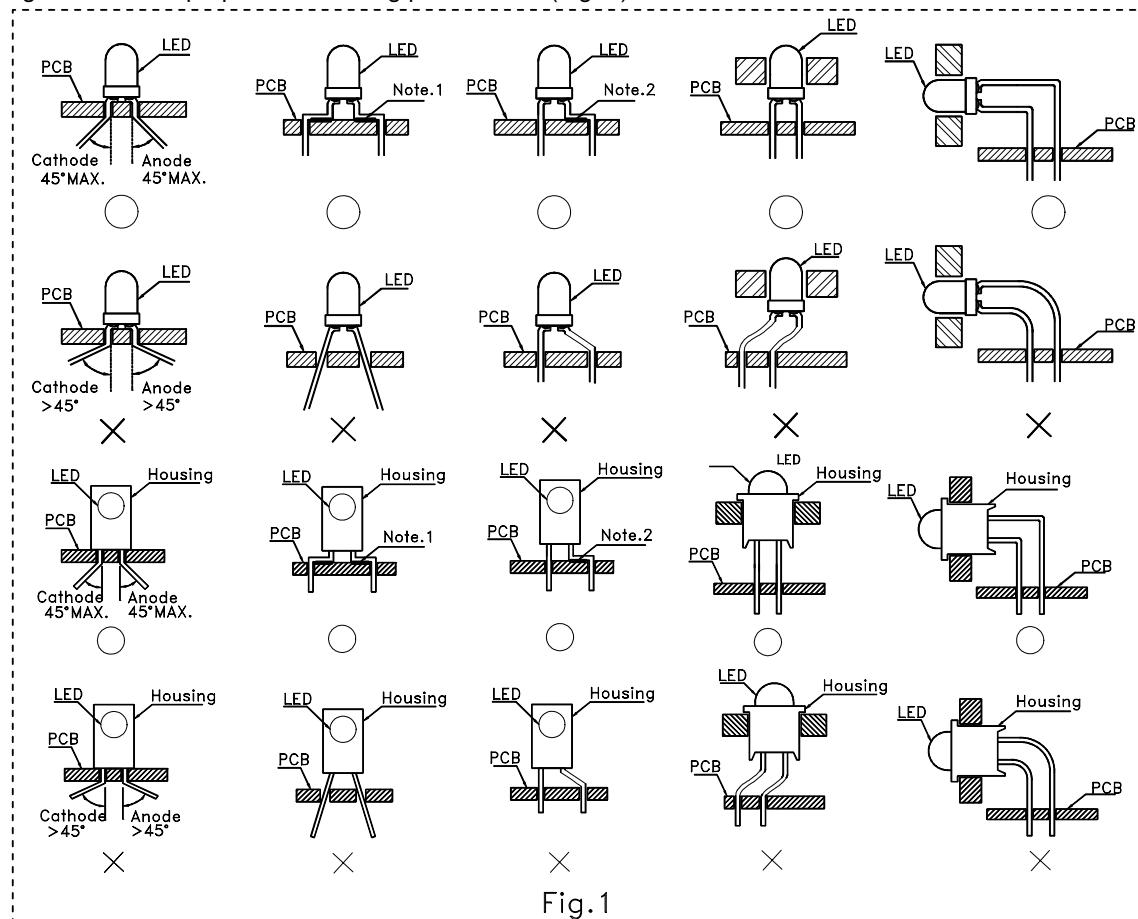
"O" Correct mounting method "X" Incorrect mounting method
