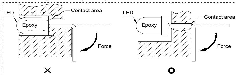
8. During soldering, component covers and holders should leave clearance to avoid placing damage stress on the LED during soldering.
