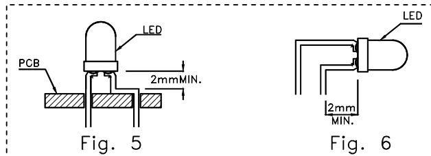
2. Lead forming or bending must be performed before soldering, never during or after Soldering.
