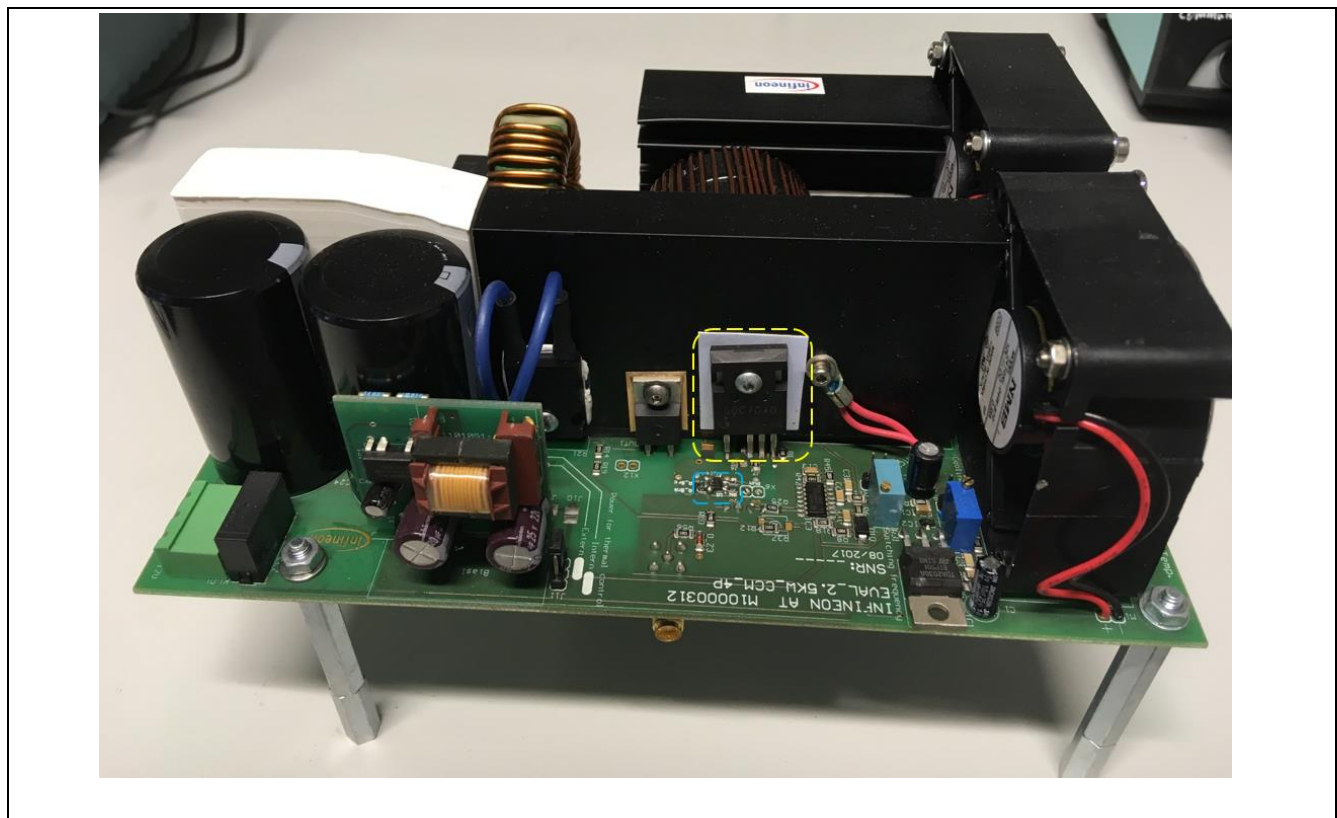
Figure 7 1EDN7550 driver in the 2.5 kW PFC evaluation board with 4-pin CoolMOS™ - Highlighted in yellow the 4-pin device and in blue the 1EDN7550B
