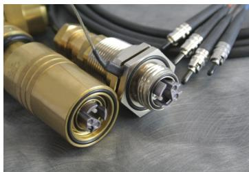
The TFOCA-II®/III® fiber optic connector is ideal for environmentally harsh conditions. The TFOCA-II® connector is designed for minimal maintenance in the field; however, if field level repair and cleaning are required, all TFOCA-II® connectors can be fully field repaired reusing all components with the exception of the termini. It has a removable end cap allowing direct access to the alignment sleeve and termini.
