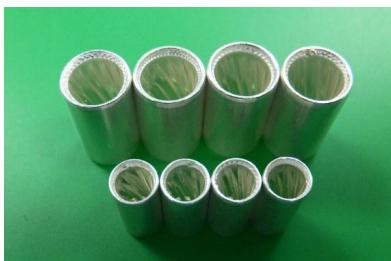
RADSOK® is a technology based upon a stamp and formed flat grid, uniquely twisted into a hyperbolic geometry to provide robust, high density contact to the mating pin contact. This patented capability allows up to 50% more current to flow through the same size terminal.
