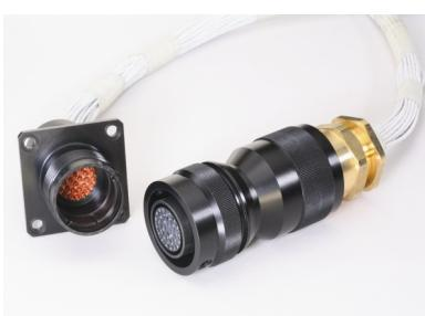
The Amphe-EX is a miniature, explosion-proof threaded connector specially designed to allow a signal to pass through Zone 1 rated areas using coax, fiber optic cables, or standard copper. Designed to meet the most severe environments, the Amphe-EX® is complimentary to Amphenol's industry-proven Star-Line-Ex. It is ATEX, IECEx, including Group I Mining Applications in Australia, GOST-R approved for the most harsh environment applications. Fiber optic custom cable assemblies available up request.
