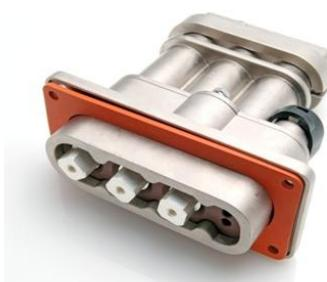
The ePower series of connectors are designed for the demanding requirement of hybrid, electric vehicle, mining, and heavy equipment markets. These connectors operate at 800V to 1000V with an amperage rating from 200A to 500A. Using the RADSOK® technology, ePower is able to offer up to a 40% smaller footprint than 3 EMI shielded cable glands used in the same end application.
