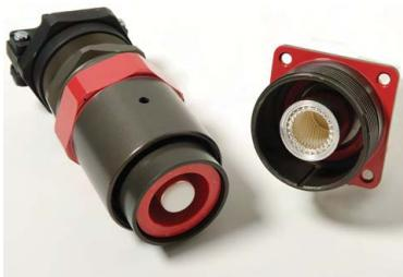
Rig-Power is a single pole power connector ranging from 925A to 1500A. The single RADSOK® contact accepts up to a 777 MCM cable, which can be sealed either with a mechanical cable clamp or cable gland. The receptacle is available with both an inline and flange mounted versions.
