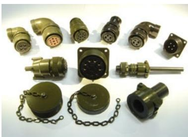
Rugged, versatile and environmental resistant connector with proven electrical capability for a less expensive solution, the 5015 series connectors are medium to heavy weight cylindrical connectors with 5 shell styles, 19 shell sizes and 5 service classes. Available in solder or crimp contacts, environmentally resistant options, threaded couplings, coaxial and thermocouple contacts, and RoHS compliant versions.
