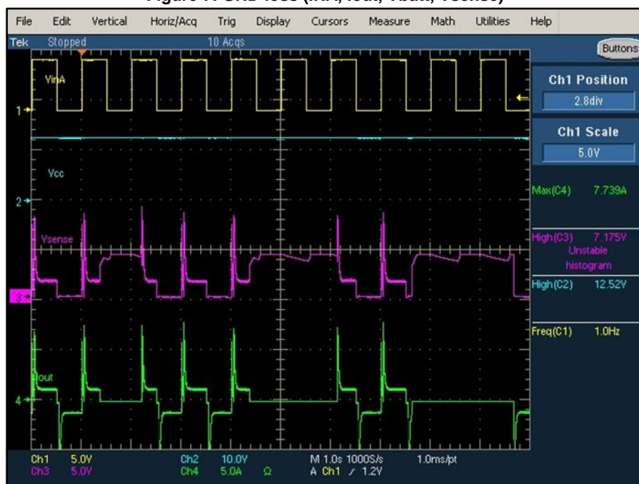
Figure 7: GND loss (INA, Iout, Vbatt, Vsense)
