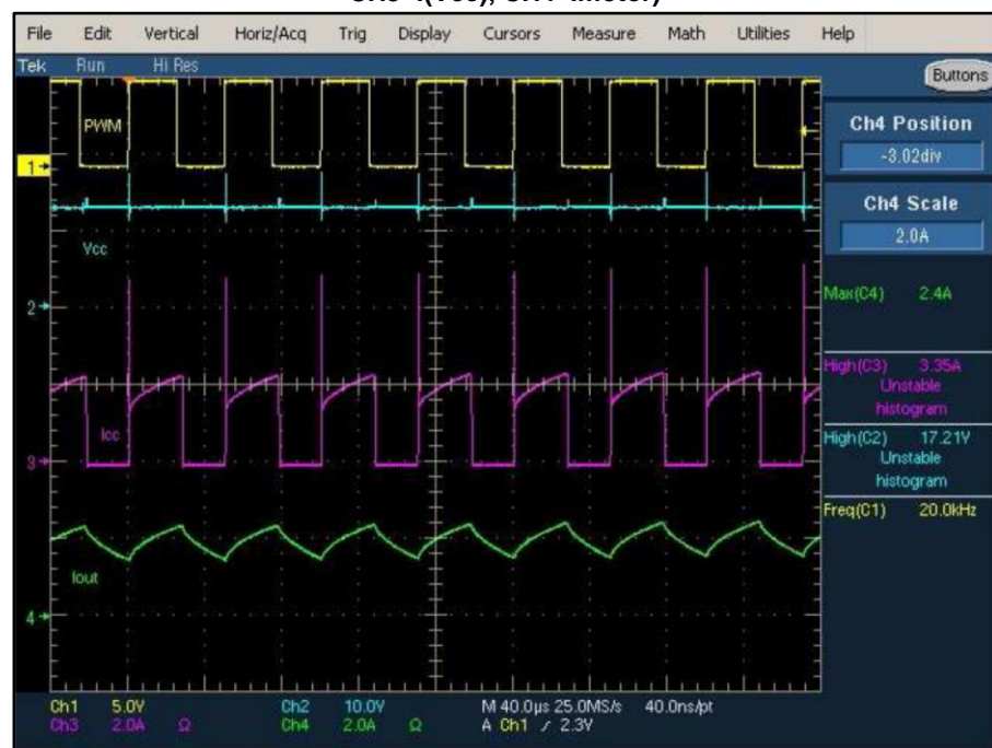
Figure 15: V_{batt}=13.5V , T_J=25^{\circ}C , Duty Cycle 50%, DC MOTOR (CH1=VPWM, CH2=Vcc, CH3=I(Vcc), CH4=Imotor)
