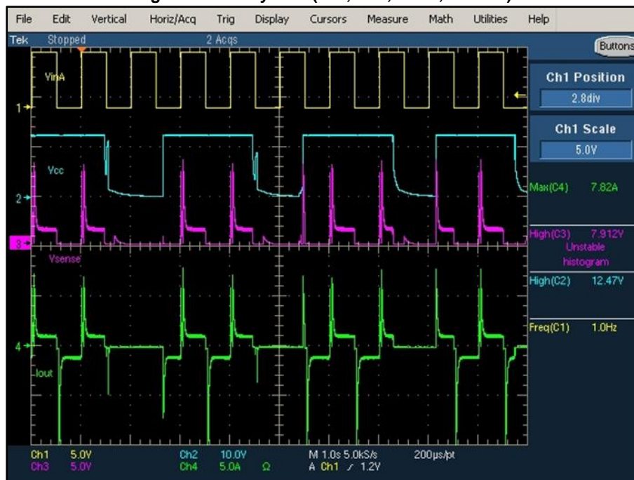
Figure 8: Battery loss (INA, Iout, Vbatt, Vsense)
