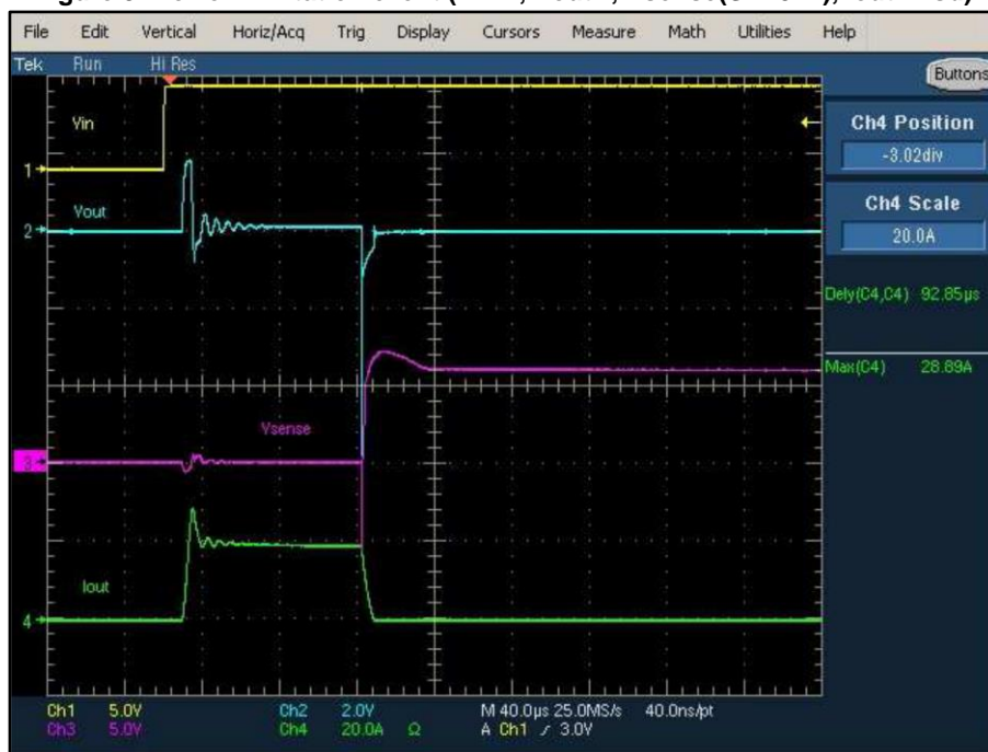
Figure 9: Power Limitation event (VINA, VoutA, Vsense(SEL0=1), Iout=Ihsd)
