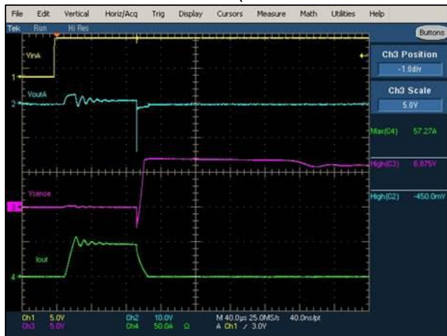
Figure 12: VN7040AY short across load event (HSA switched on while LSB is already ON)
