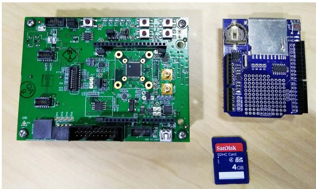
Figure 1. Required Boards: EVAL-ADuCM3029 EZ-KIT Evaluation Board (Left), Arduino-Compatible SD Card Shield (Top Right), SD Card (Bottom Right)
