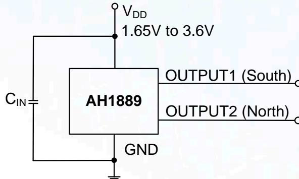
Note:  $C_{IN}$  is for power stabilization and to strengthen the noise immunity, the recommended capacitance is 100nF typical.
