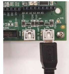
Figure 21. USB to UART Connection
