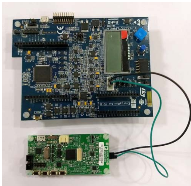
Figure 32. Board Setup for Measuring the Score
