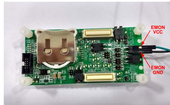
Figure 29. Board Setup for Downloading the Code
