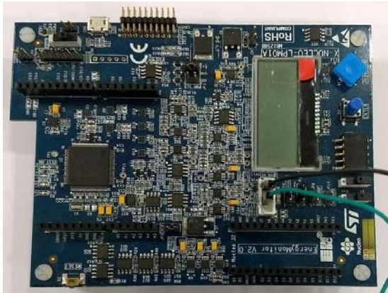
Figure 27. EEMBC EnergyMonitor Hardware
