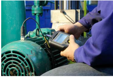
Figure 2. Existing Manual Probe Methods for Equipment Vibration Shift Monitoring Lack Repeatability and Reliability
