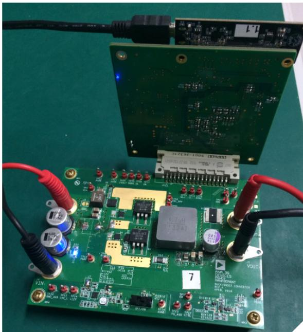
**Efficiency:** the efficiency of the demo board is ~90% at its maximum rating, with 20 A CC mode for both charge and discharge with a 3.3 V load. To achieve this number, the external diode, shunt resistor, inductor, and MOSFETs are optimized. ADP1974 is also evaluated on this demo board, and the synchronizing mode helps the system efficiency to go up to 96%.
