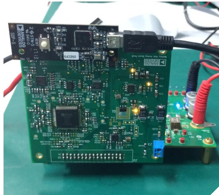
(0 A to 20 A), short term stability (noise), and CMRR over the full voltage range (0 V to 3.6 V). The typical current accuracy of the ADI solution verified on a demo board is less than 0.01% under 25°C ( $\pm 10^\circ\text{C}$ ). A similar analysis can be performed for voltage accuracy, which is also less than 0.01% verified on this demo board.
