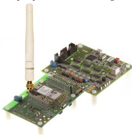
Figure 1 DC9018B Mote (left) connected to the DC9006A Interface Card (right)
