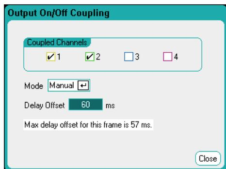
Under Coupled Channels, select the outputs that will be coupled. Outputs excluded from an output on/off delay sequence can be put to other uses. Turning the output on or off on any coupled output will cause all coupled outputs to turn on or off according to their user-programmed delays.
