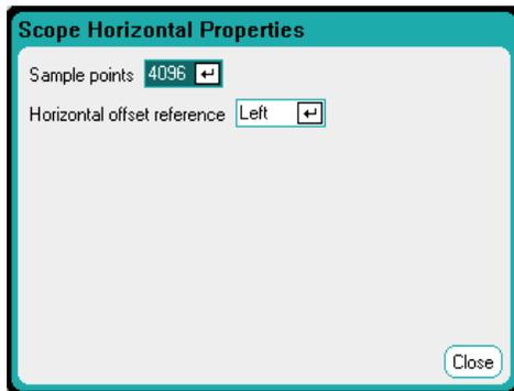
**Sample Points** - lets you specify the number of points in a scope trace. The maximum number of points that can be specified depends on the number of scope traces that have been enabled. The minimum number of points that can be specified is 1024.
