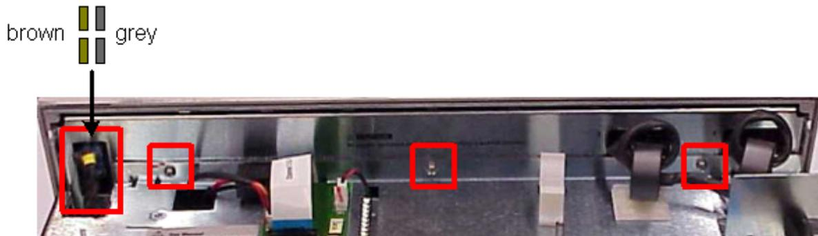
**Step 6.** Remove two screws using a T10 from each side of the front panel.
