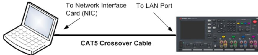
1. Connect the instrument to the computer using a LAN crossover cable. Alternatively, connect the computer and the instrument to a standalone hub or switch using regular LAN cables.
