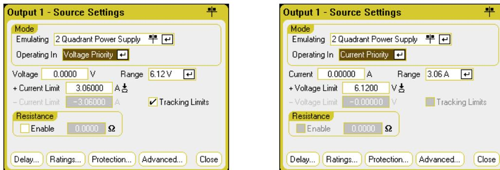
**Operating in** – selects either Voltage Priority or Current Priority. The other settings in 2-quadrant mode are the same as the settings in 4-quadrant mode except that you cannot program negative voltages or negative voltage limits. Because of this, voltage tracking is not available in Current Priority mode. Note that the negative voltage limit is fixed at  $-10$  mV. Refer to [N678xA Multi-Quadrant Operation](#) for a detailed description of voltage and current priority.
