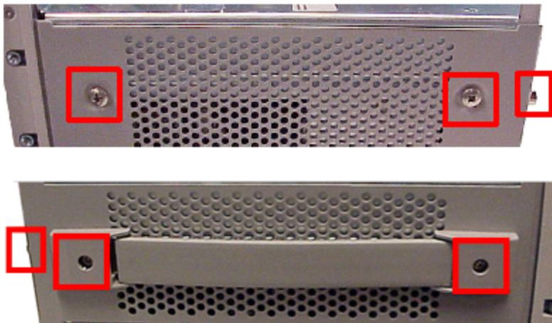
**Step 3.** Remove three screws using a T10 driver from the rear panel.
