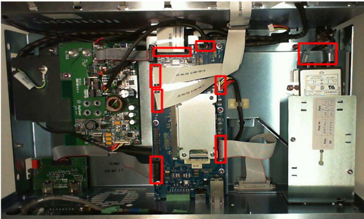
**Step 5.** Unhook the cable tie from the bulk shroud and remove four screws using a T20 driver. (Figure shows PCA boards removed for clarity)
