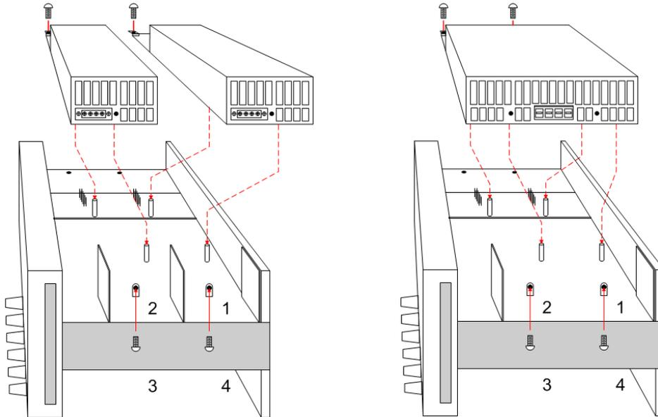
The location of the power modules inside the mainframe determines their front panel output and programming channel assignments. For example, modules installed in channel 1 will be connected to the wire harness for output 1. Modules installed in channel 4 will be connected to the wire harness for output 4.
