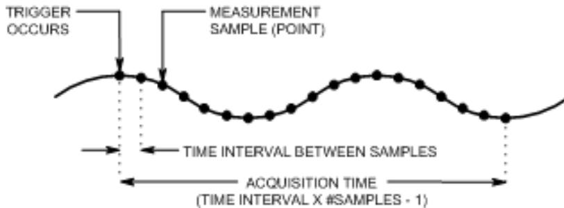
You can vary the measurement data sampling rate using the following commands. For example, to set the time interval to 60  $\mu$ s with 4096 samples, use:
