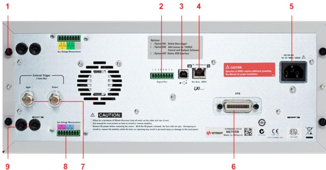
1. **Cover screw** - Facilitates top and bottom cover removal for power module installation.
