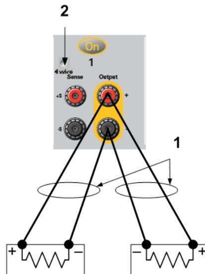
This minimizes mutual coupling effects and takes full advantage of the power module's low output impedance. Keep each wire-pair as short as possible and twist or bundle the wires to reduce lead inductance and noise pickup. The goal is to always minimize the loop area or physical space between the + and - load wires from the power analyzer to the load. Keep the load leads under 14.7 meters (50 feet) per lead because of inductance effects
