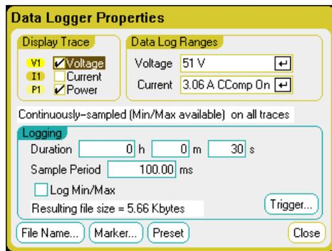
**Display Trace** - lets you select which traces to display for the output. If no box is checked, no data logging will occur on the output.
