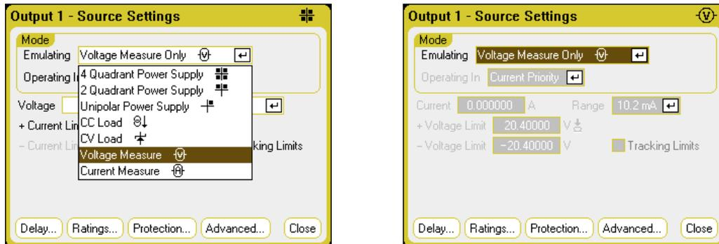
**Voltage Measure** - the Voltage Measure mode works best when the sense terminals are connected to the output terminals. You can use 4 Wire sensing and connect the sense and output leads directly to the DUT as shown below, or you can use Local sensing and connect only the output leads to the DUT.
