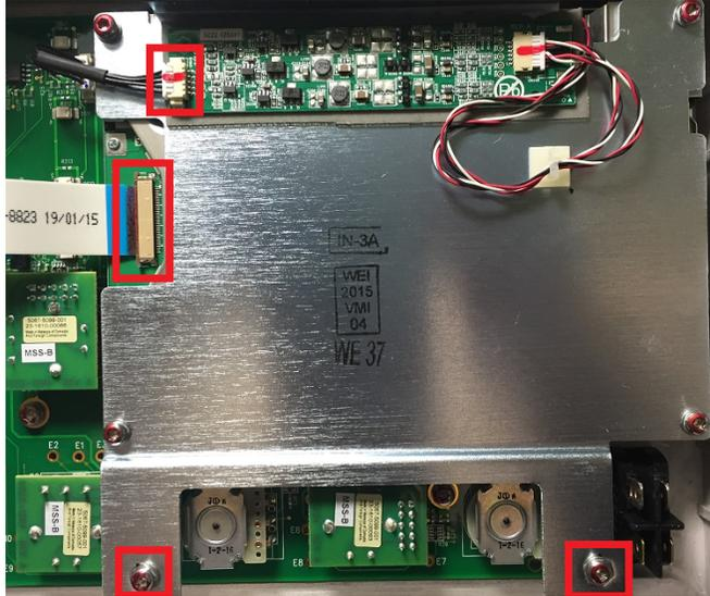
**Step 3.** Disconnect one cable and remove four screws using a T10 driver to remove display from bracket.
