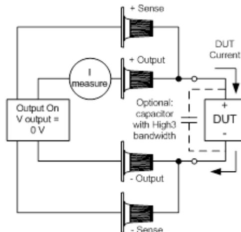
When the Measure Only modes are selected, the output is enabled and the voltage or current measurement is continuously displayed on the Meter View. Both voltage and current meters are active in either mode.
