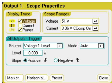
**Display Trace** lets you select which traces to display for the output. If no box is checked, no traces will be displayed for that output. Voltage, current, and power traces can be displayed simultaneously only on Models N676xA and N678xA SMU, as these models have simultaneous voltage and current measurement capability (see [Model Differences](#)). All other power modules can display either voltage or current traces, but not simultaneously.
