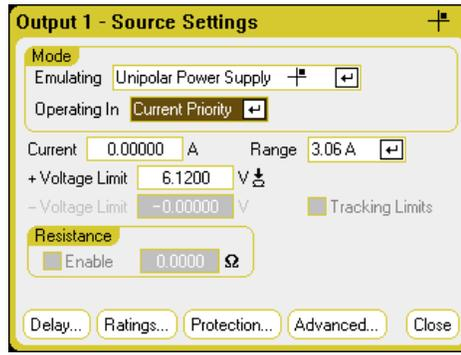
**Resistance** - This is only available on Keysight N6781A and N6785A. Output resistance programming is primarily used in battery emulation applications, and only applies in Voltage Priority mode. Values are programmed in Ohms, from  $-40\text{ m}\Omega$  to  $+1\ \Omega$ .
