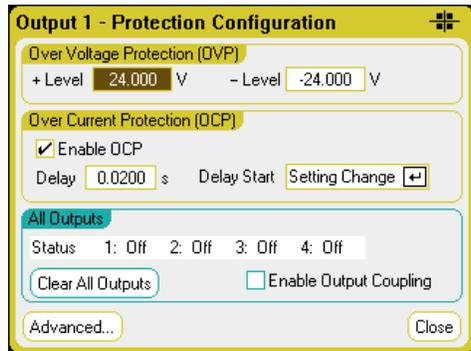
**Over Voltage Protection** - Over-voltage protection disables the output if the output voltage reaches the OVP level. To set the over-voltage protection, enter an over-voltage value in the +Level field.
