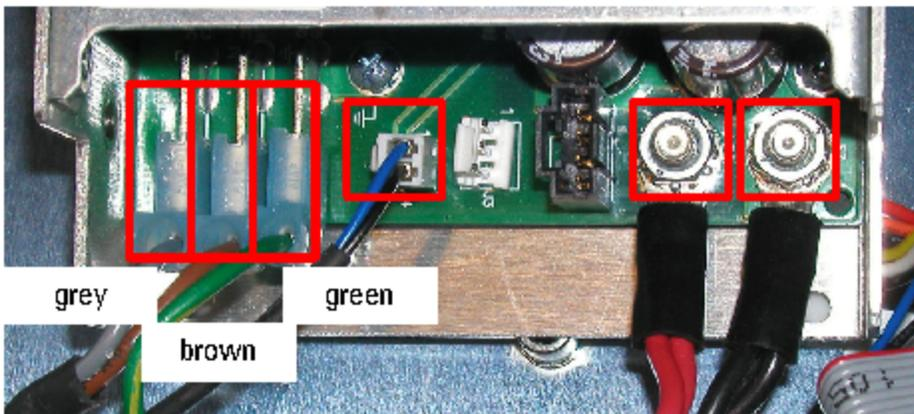
**Step 6.** Remove the bulk supply.
