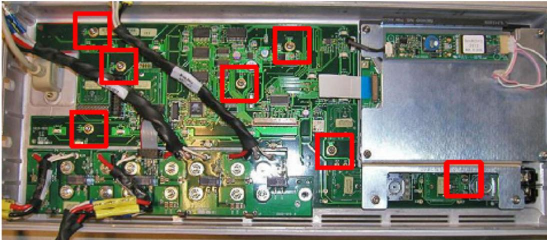
**Step 4.** Remove the seven knobs from the front panel.
