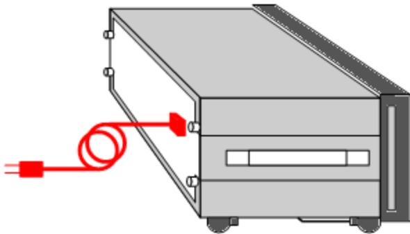
The AC input on the back of your unit is a universal AC input. It accepts nominal line voltages in the range of 100 VAC to 240 VAC. The frequency can be 50 Hz, 60 Hz, or 400 Hz.
