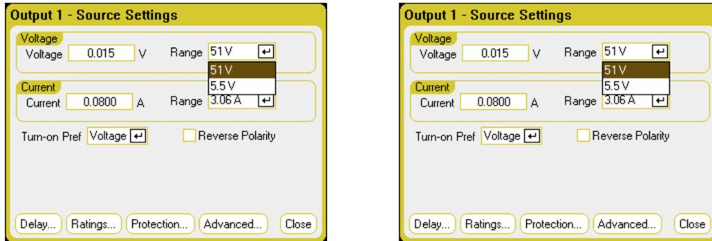
**Voltage or Current Range** – For outputs with multiple ranges, you can select a lower range if you need better output resolution. Use the navigation keys to highlight the Range field. Press the Enter key to access the dropdown range list. Use the navigation keys to select the desired output range.
