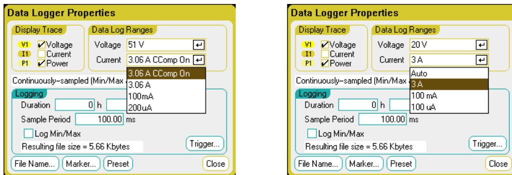
Some models have a high measurement range labeled CComp On, which is selected by default. The CComp On range compensates output current measurements during voltage transients. For more information, see [Dynamic Current Measurement Control](#).
