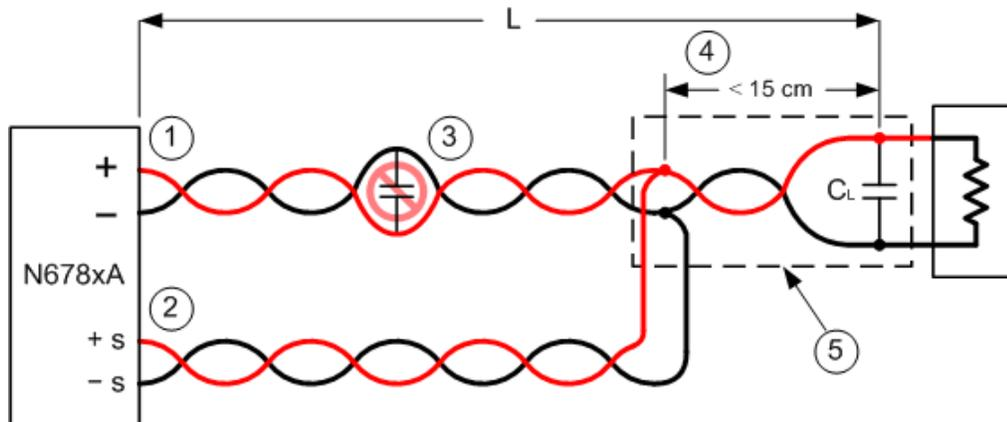
1. Load wires must be twisted-pair or coax and must not be twisted along with the sense wires. Refer to the above table for length (L).
