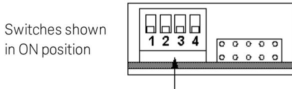
**CAUTION** Do not use a pencil to move the switches. Any graphite dust that gets on the switches will conduct electricity.
