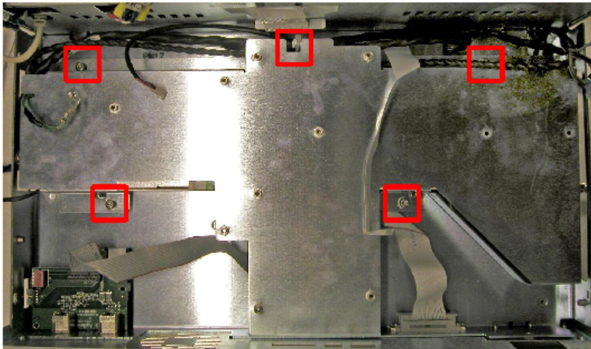
**Step 6.** Gently lift bulk shroud out of mainframe and place on right side of mainframe (non-handle side - right side when viewed from front).
