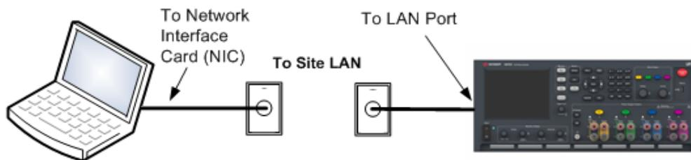
1. Connect the instrument to the site LAN or to your computer using a LAN cable. The as-shipped instrument LAN settings are configured to automatically obtain an IP address from the network using a DHCP server (DHCP is set On). The DHCP server will register the instrument's hostname with the dynamic DNS server. The hostname as well as the IP address can then be used to communicate with the instrument. The front panel **lan** indicator will come on when the LAN port has been configured.
