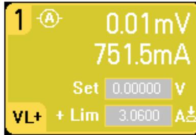
When the Measure Only modes are selected, the output is enabled and the voltage or current measurement is continuously displayed on the Meter View. Both voltage and current meters are active in either mode.
