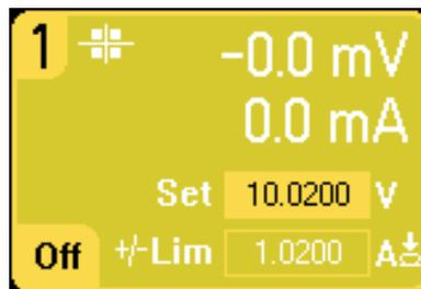
Lastly, you can press the **Settings** key to access the Source Settings window. Use the navigation keys to highlight the Voltage or Current fields. Then enter the voltage and current values with the numeric
