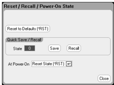
Selecting Reset to Defaults lets you immediately return the instrument to its factory default settings as described under **Reset State**.
