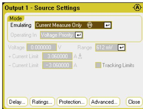
The following additional settings are also required. Remote sensing (4 Wire) is always required. For applications with transient voltage drops, use the High3 setting with a compensation capacitor across the DUT. Capacitors can be film or ceramic with values from 7  $\mu\text{F}$  to 150  $\mu\text{F}$ . Refer to [Keysight N678xA SMU Wiring](#) for additional wiring information.
