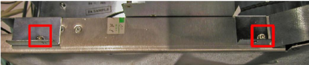
**Step 5.** Disconnect four connections and remove two 11/32 in. nuts from the bulk supply.
