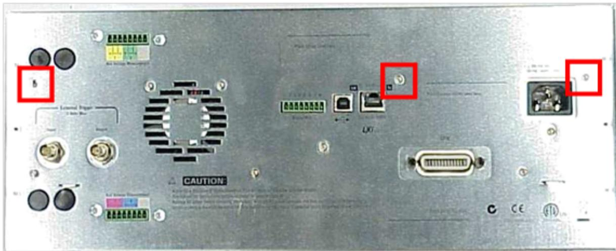
**Step 4.** Remove three screws using a T10 driver from the front panel sub assembly.
