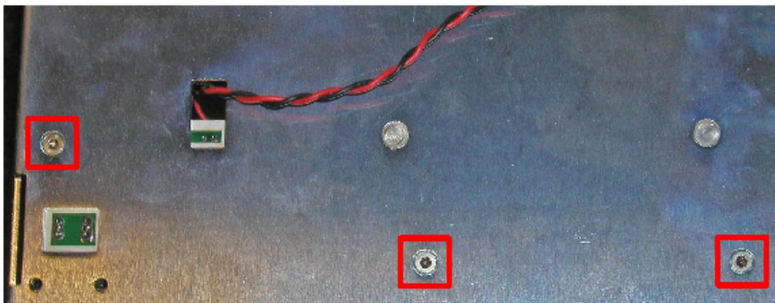
**Step 3.** Disconnect any remaining cables if required, and either cut or carefully slide the two push-on retainers off of the retaining pins.
