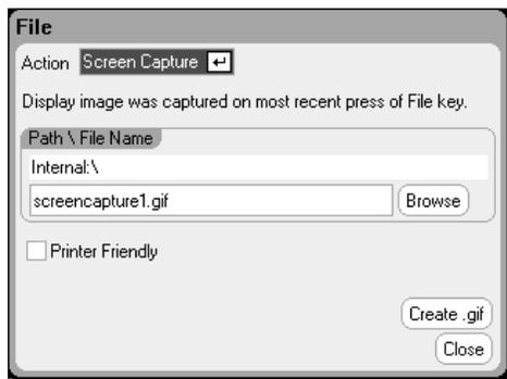
A copy of the current screen is saved whenever the **File** key is pressed.
