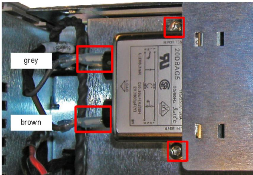
**Step 4.** Remove the AC Module
