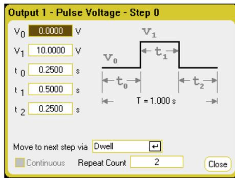
Press the Advanced button to specify what happens when the Arb sequence completes – select whether the output Returns to the DC Value that was in effect before the waveform started, or whether the output should remain at the Last Arb Value. Also specify if the Arb sequence should repeat, either continuously or only for a specified repeat count. A repeat count of 2 runs the sequence twice.
