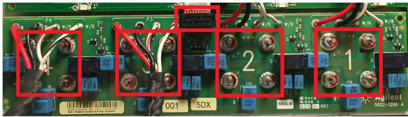
**Step 3.** Remove the binding post board.
