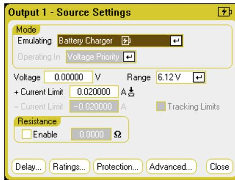
**Battery Emulator** - lets you specify the battery voltage and range as well as the + and - current limits. The output resistance is programmable, from  $-40\text{ m}\Omega$  to  $+1\ \Omega$ . Voltage Priority mode is locked. The voltage setting is limited to positive values. The + and - current limits are set to their maximum values. The - current limit setting sets the current limit when the battery is being charged.
