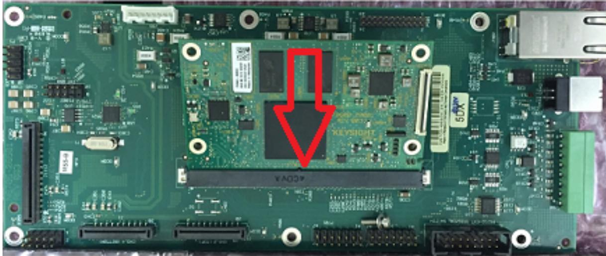
**Step 5.** Then position the heat spreader over the board and gently push the heat spreader down. Install the four screws.
