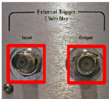
**Step 3.** Remove the BNC board
