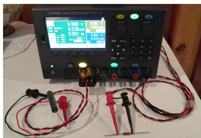
It is good engineering practice to twist your wires to reduce lead inductance and reduce noise pickup. In the test example shown above, Channel 1 is set up for 2-wire operation using a single twisted pair. Channel 2 is set up for 4-wire operation using a twisted pair for the output leads and a separate twisted pair for the remote sense leads.
