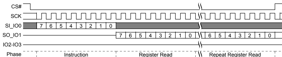
Figure 11.12 Read Configuration Register (RDCR) Command Sequence
