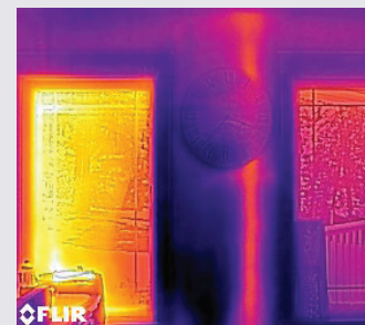
Warm Drain Pipe in Wall
