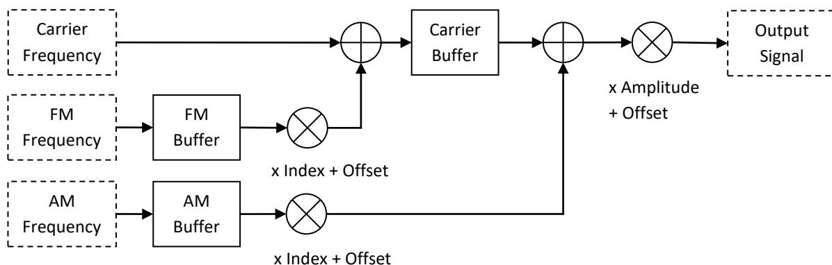
The Carrier/FM/AM nodes can be configured by selecting with the AnalogOutNode constants.
