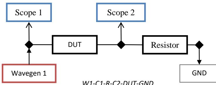
The DUT (Device Under Test) stands for the inductive or capacitive load to be analyzed and Resistor is the reference resistor. The resistor value depends on the load value and frequency.
