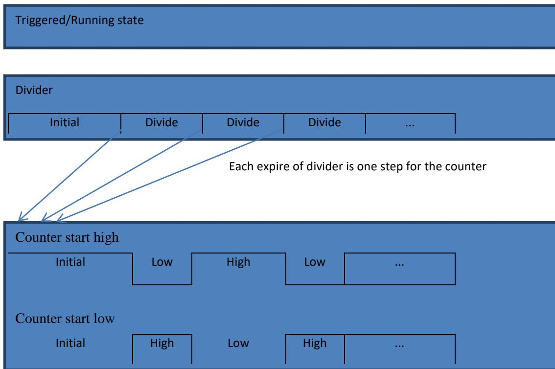
For pulse signal the initial level and initial value are specified with *FDwfDigitalOutCounterInitSet* function. These are loaded when entering Running state.
