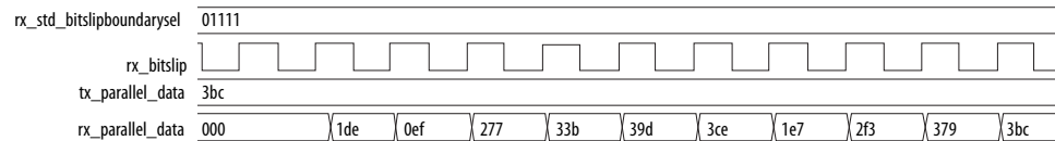
Figure 141. RX Bit Slip in 16-bit Mode
