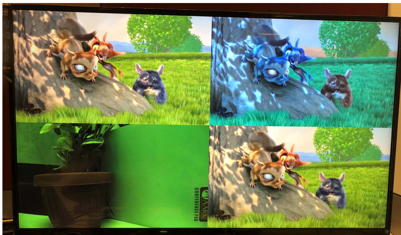
Figure 3-18: Multi-Stream—3 HDMI and 1 MIPI Input Sources @ 1080p60
