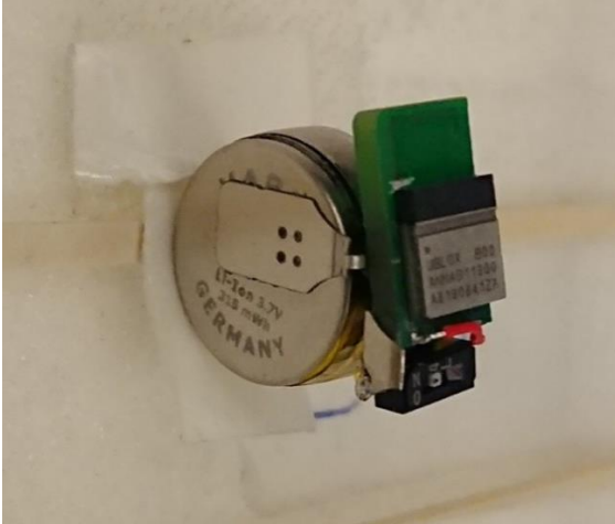
Figure 38: A tiny ANNA-B1 application including coin cell battery
