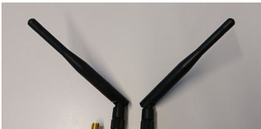
Figure 2: Example of orthogonally polarized dipole antennas
