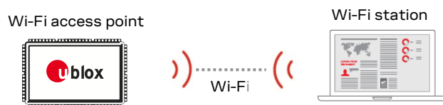
Figure 5: Wi-Fi access point connection
