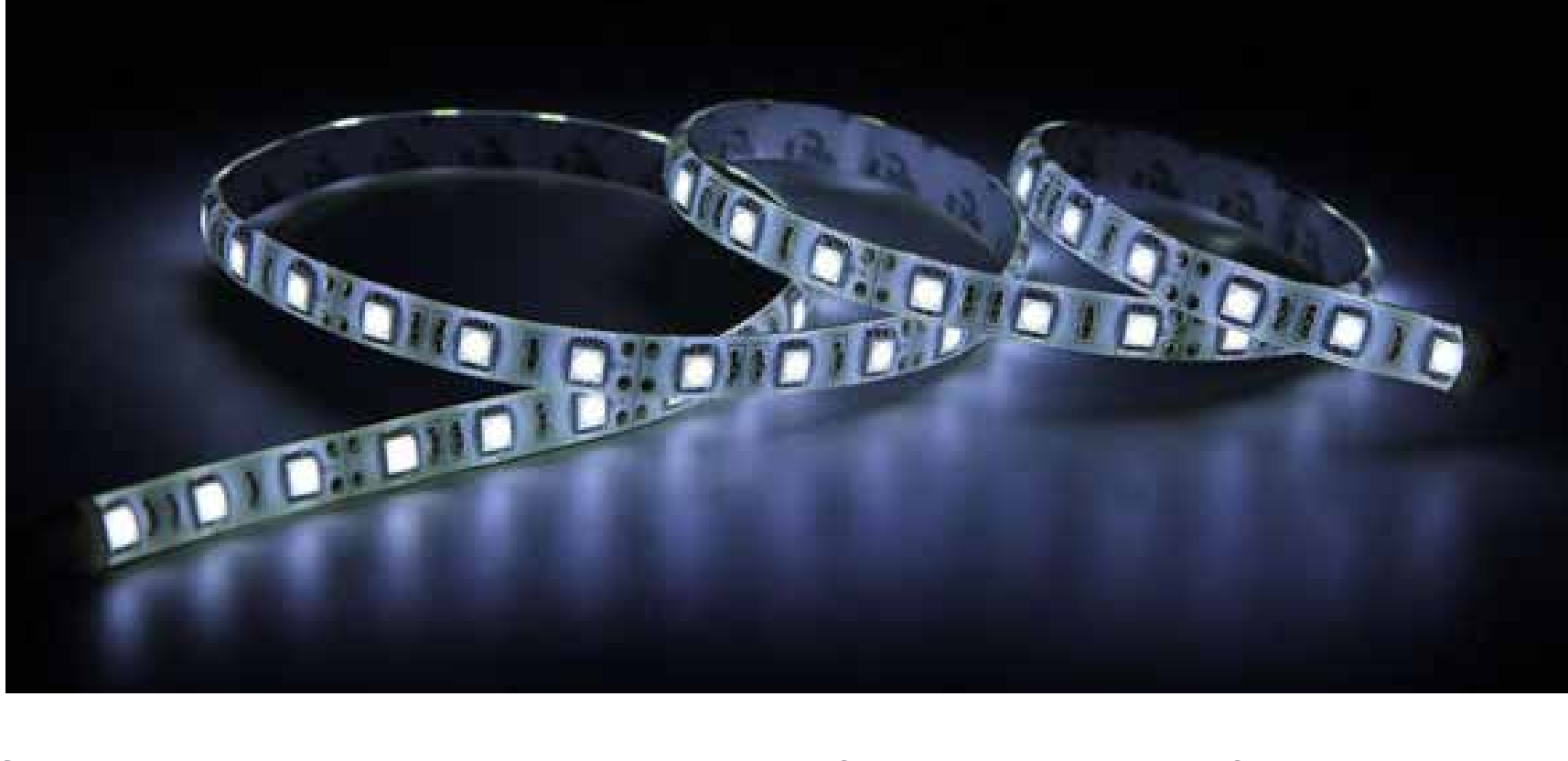
Figure 1: LED light strips consist of narrow, flexible circuit boards populated with surface-mount LEDs of various colors. With a built-in IC, individual RGB LEDs on the light strip will be independently addressable.
