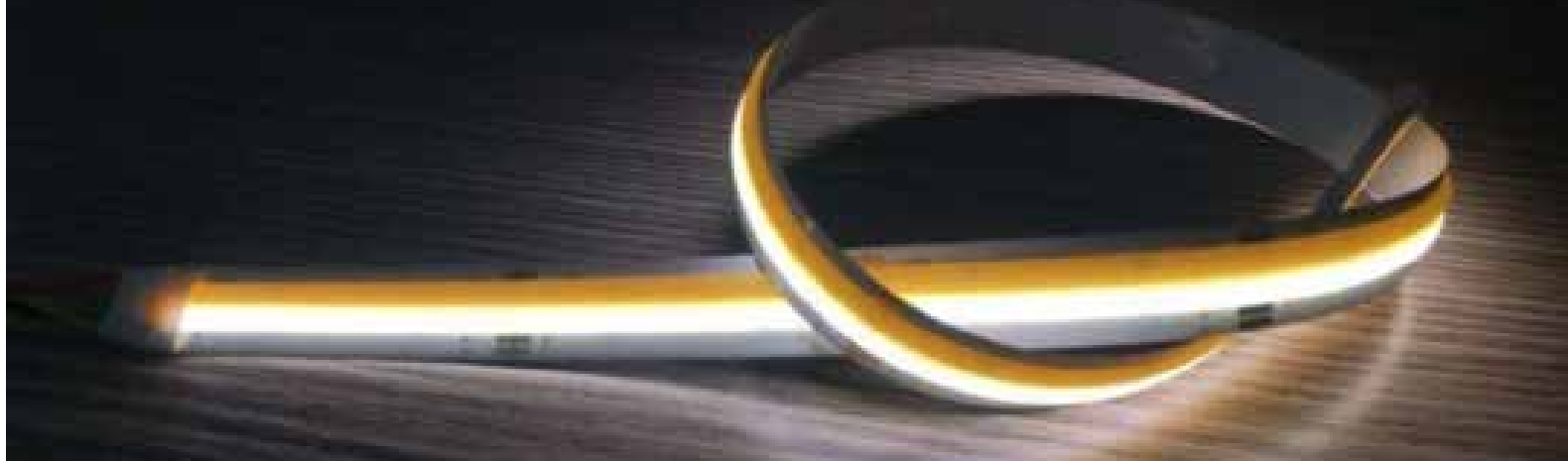
Figure 3: Chip on board (COB) light strips consist of unpackaged LEDs mounted to the flexible circuit board strips. They can generate very high luminous flux densities.
