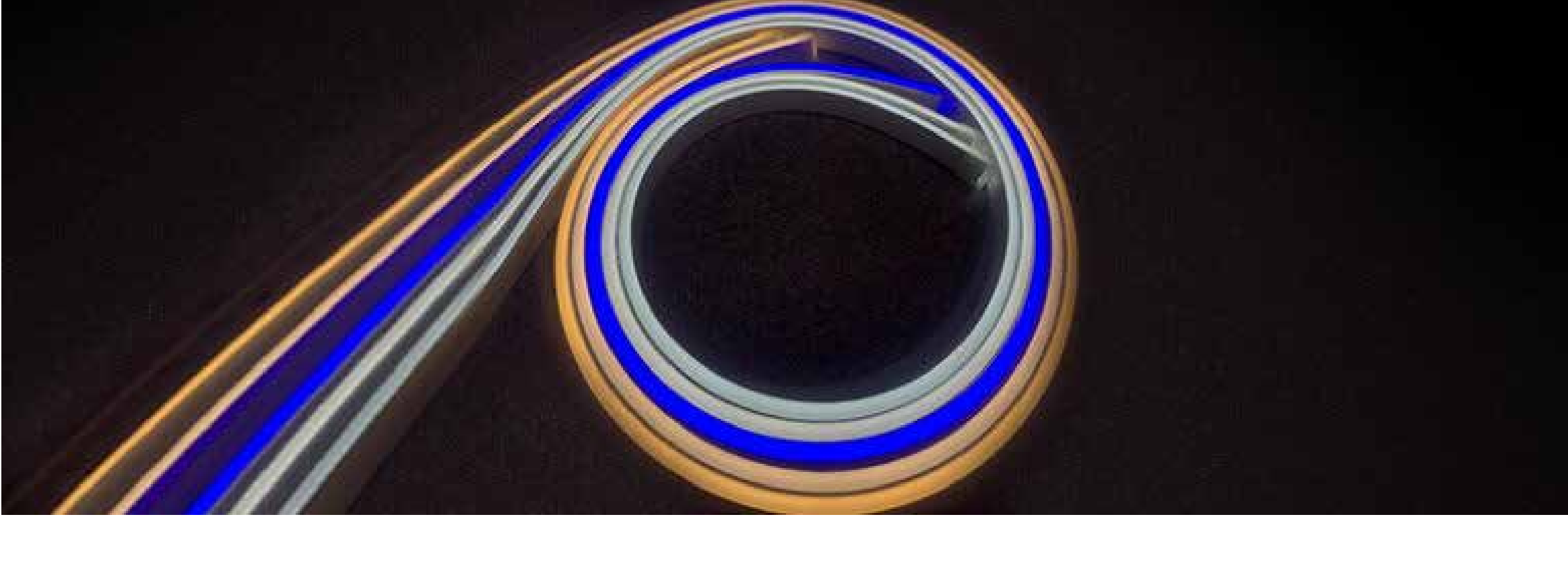
Figure 2: In rope lights, the LEDs are encased in silicone tubes that can be transparent or mixed with diffusing material. Here, too, individual LEDs can be independently addressable and color tuned in real time for sophisticated effects.
