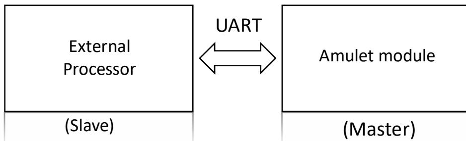
In this system the Amulet module is setting and reading variables stored in the external processor. For the Amulet module to operate in master mode, the slave processor needs a memory space allocated that maps the VDP-RAM. The slave protocol is straightforward; a code example of the CRC protocol is available in C++.
