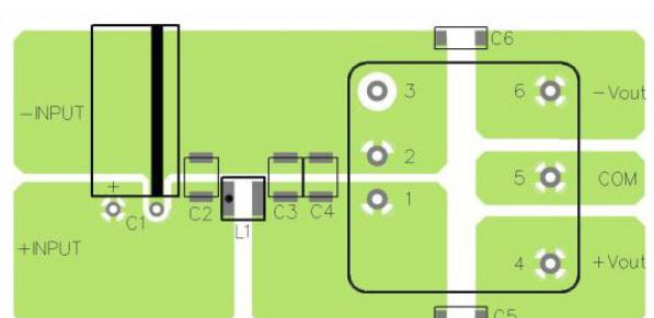
**Suggested components to comply with EN 55032 Conducted and Radiated Emissions Class B limits**
