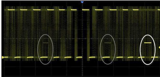
With a waveform update rate of up to 200,000 wfm/s, the oscilloscope can easily capture unusual or low probability events. In Sequence mode, the waveform capture rate can reach 890,000 wfm/s.
