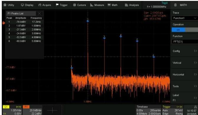
Hardware-accelerated FFT supports up to 4 Mpts operation. This provides high-frequency resolution with a fast refresh rate. The FFT function also supports a variety of window functions so that it can adapt to different spectrum measurement needs. Three modes (Normal, Average, and Max hold) can satisfy different requirements for observing the power spectrum. Auto peak detection and markers are supported.
