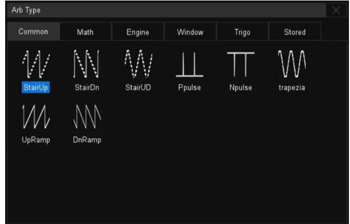
The 50 MHz waveform generator can output waveforms with up to 50 MHz frequency and  $\pm 3$  V amplitude. Six basic waveforms plus multiple types of arbitrary waveforms are built-in.
