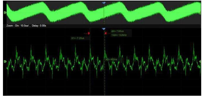
Using hardware-based Zoom technique and record length of up to 400 Mpts, users can select a slower time-base without compromising the sample rate, and then quickly zoom in to focus on the area of interest.
