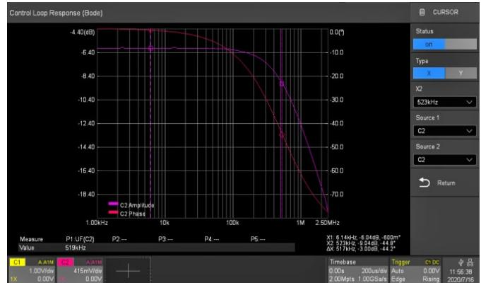
The oscilloscope can control the built-in waveform generator or a stand-alone Teledyne Test Tool generator, to scan the amplitude and phase-frequency response of the DUT, and display the data as a Bode Plot. This makes it possible to replace expensive network analyzers in some applications.
