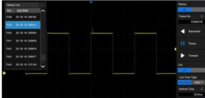
History function can record up to 80,000 frames of waveforms. The recording is executed automatically so that the customer can playback the history waveforms at any time to observe unusual events and quickly locate the area of interest using the cursors or measurements. The failed frames of the Mask Test can be stored as history.
