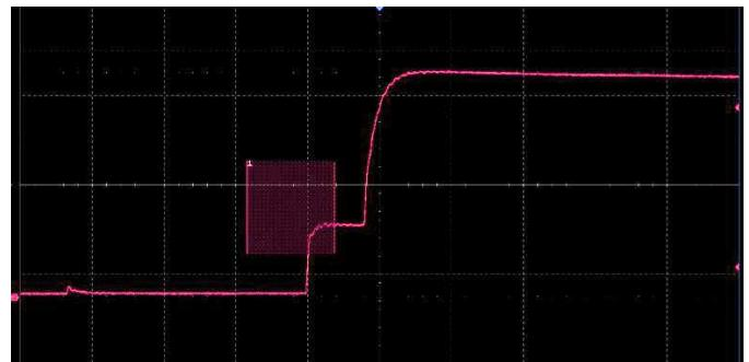
Trigger Zone is available for advanced triggering. Combine spatial triggering with common trigger mode to isolate signals of interest.
