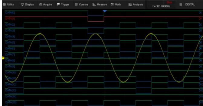
Four analog channels plus 16 digital channels enable users to acquire and trigger the waveforms then analyze the pattern, simultaneously with one instrument.
