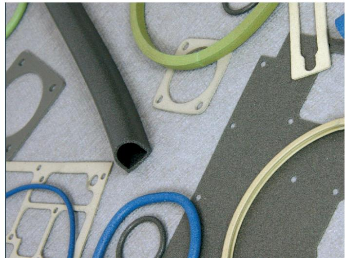
Conductive elastomers are fully cured silicones or fluorosilicone loaded with electrically conductive particles providing superior electromagnetic interference/radio frequency interference (EMI/RFI) shielding performance combined with excellent environmental sealing. The various conductive fillers are designed to ensure galvanic compatibility whilst providing low contact resistance between mating surfaces.
