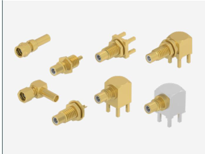
TE Connectivity (TE) introduces an extension of our SMC connector RF product line. SMC connectors are miniature and lightweight, designed for use in critical applications where limited space and vibration are of major concern. These connectors have a constant impedance of 50 Ω, a voltage rating of 350 volts, and operate at frequencies up to 10 GHz. SMC connectors have a threaded coupling and can be used with a wide range of miniature coaxial cable sizes including RG 174, 188A, and 316.
