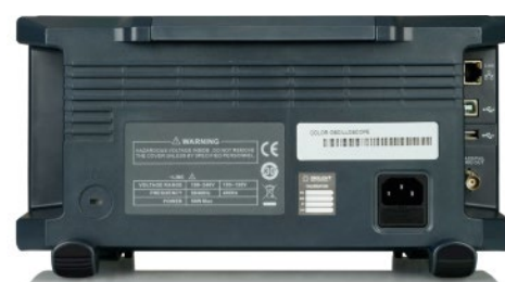
Back panel of T3DSO1104, T3DSO1202A, T3DSO1204, T3DSO1302A
