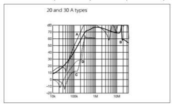
For example, the figure above shows the filter attenuation plot of a Schaffner FN350 Compact EMC/RFI filter for motor
