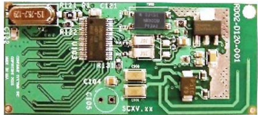
26mm x 59mm CX86500 Modem Reference Design
