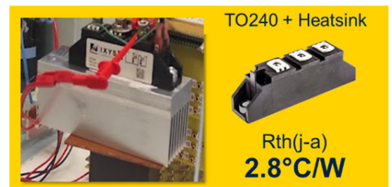
Figure 5. Junction to ambient thermal impedance
