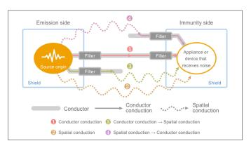
Aside from ensuring that the leads are adequately attached to the appropriate connection points and that the shielding is effectively connected, there are a limited number of methods to ensure that noise produced by the device won't be emitted from the leads and external noises will not be conducted into the device through the leads. EMI suppression filters are one of the most common and effective ways of attenuating noise and interference signals.
