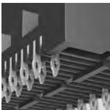
Staggered press-fit tails
