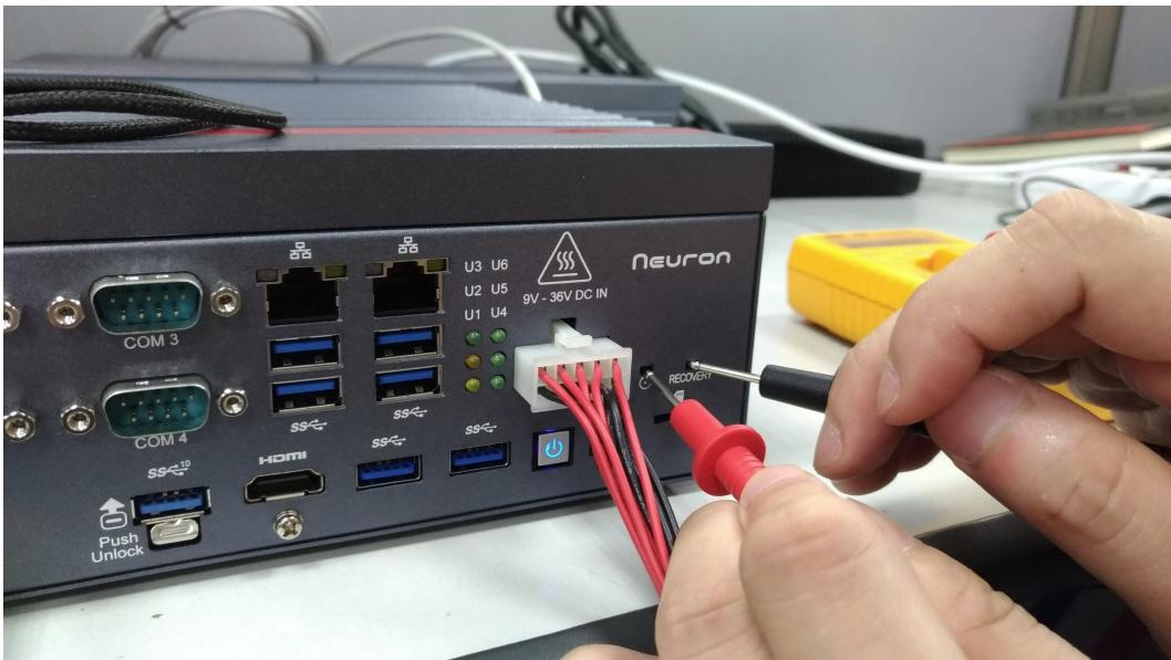
iii) Release RESET button first and then release RECOVERY button.
