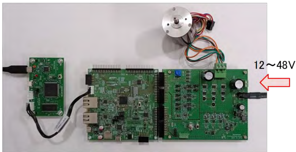
Figure 4-10 Power supply from DC jack
