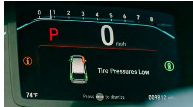
New vehicles have included factory installed dTPMS solutions for the past years, with a wireless connection from the wheel to a central control unit. The wireless technology used in these solutions will be a sub-GHz proprietary protocol. These solutions give you a warning when the tire pressure drops below a set threshold and can show the pressure for each wheel/tire on the dashboard display screen.
