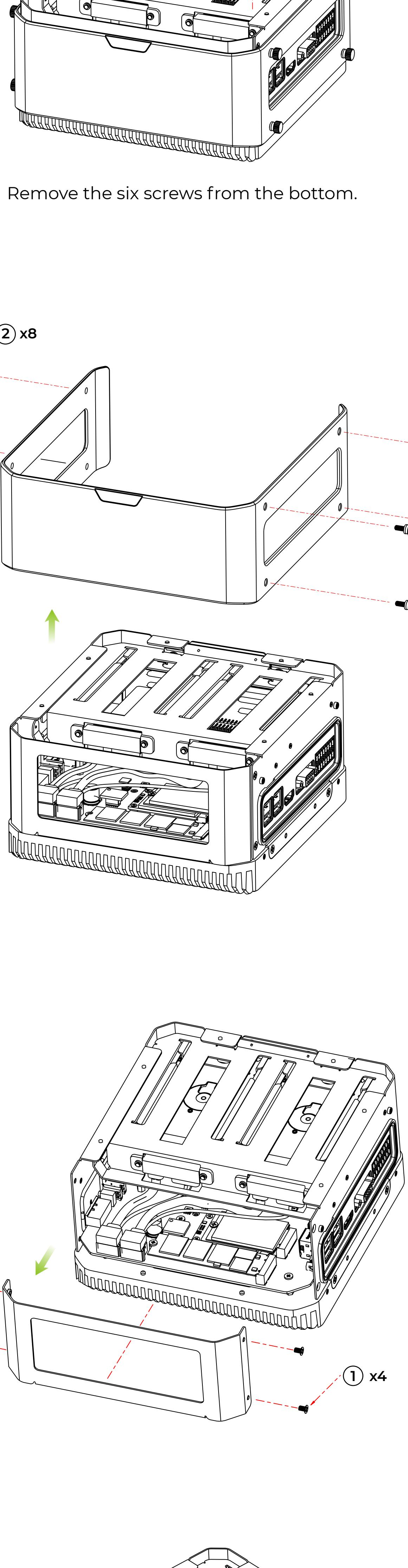
Remove the six screws from the bottom.
