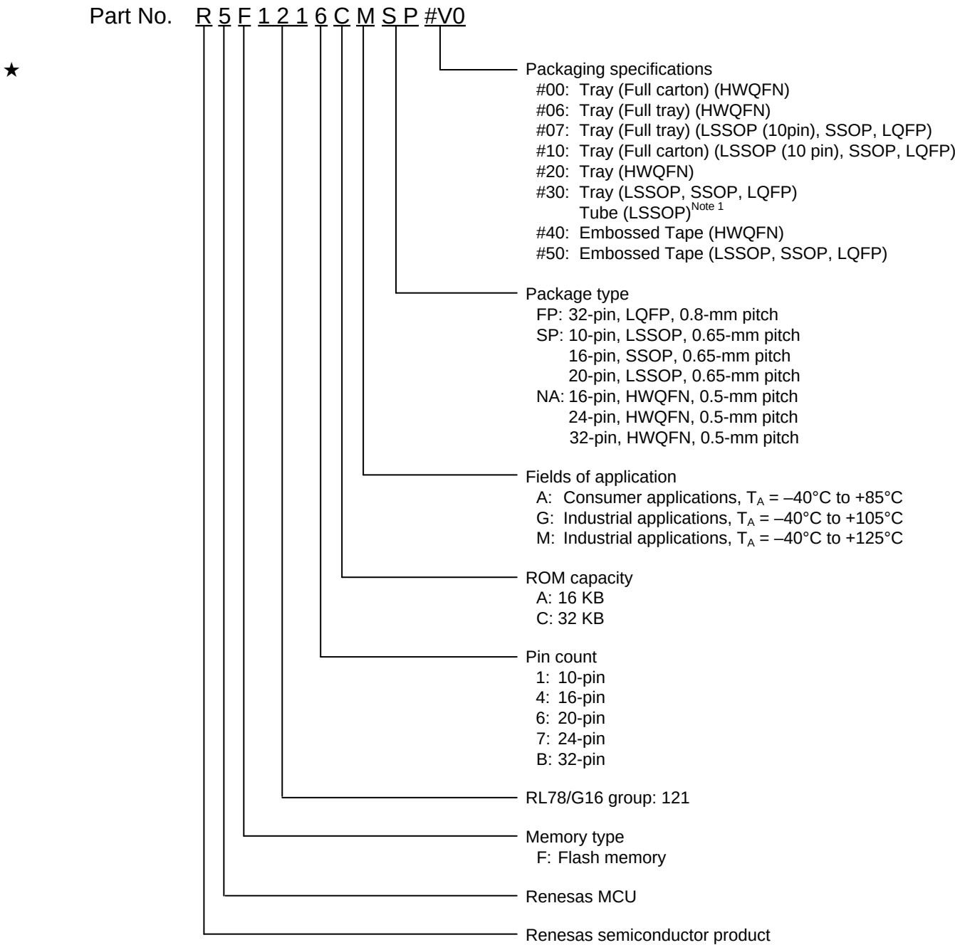
Figure 1-1. Part Number, Memory Size, and Package of RL78/G16
