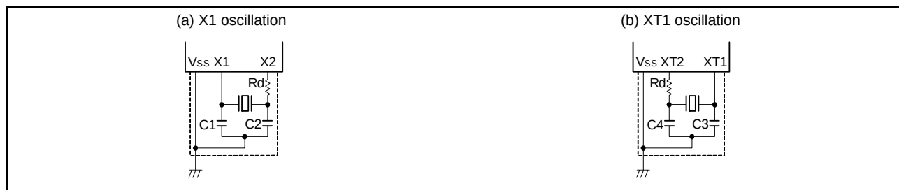
Figure 6 - 23 Examples of External Circuits
