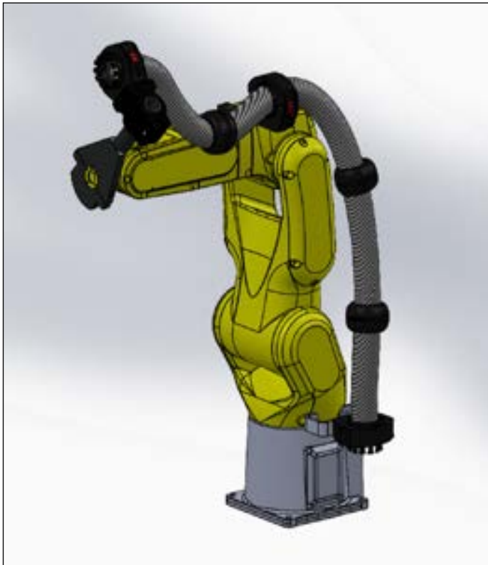
40.48.001.01 Complete robotic dresspack, Axis 1-6, without retraction system, high-flex conduit with ID 46.3mm
