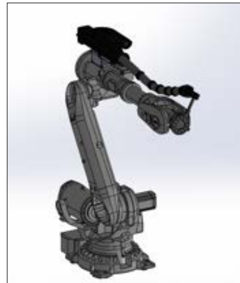
26.70.321.01 Complete robotic dresspack, Axis 3-6, TecBox retraction system, 600mm stroke, high-flex conduit with ID 64mm
