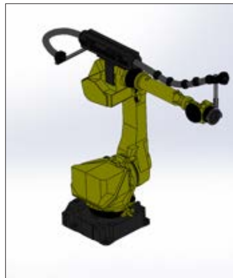
11.70.121.01 Complete robotic dresspack, Axis 3-6, TecLiner retraction system, 350mm stroke, high-flex conduit with ID 64mm
