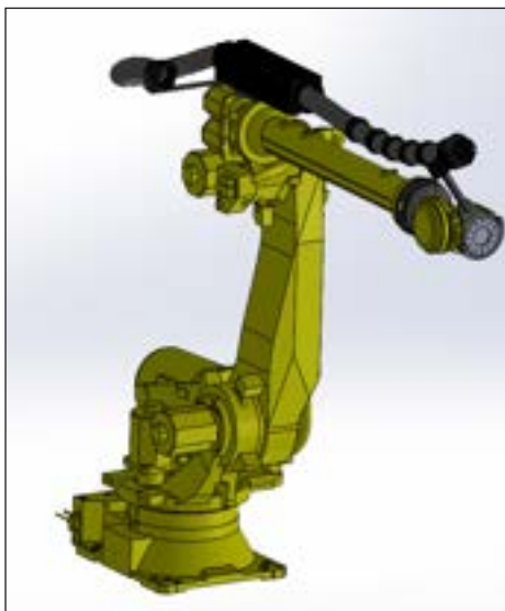
22.70.121.01 Complete robotic dresspack, Axis 3-6, TecLiner retraction system, 350mm stroke, high-flex conduit with ID 64mm
