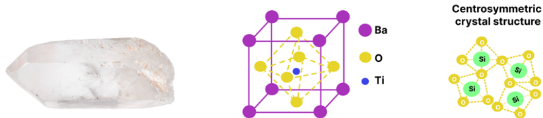
Figure 1: Natural piezoelectric crystals, engineered piezoelectric ceramics, and non-piezoelectric structures demonstrate the variety of materials used in piezoelectric applications. (Sources: (a) Ekaterina/stock.adobe.com, (b, c) Mouser Electronics)
