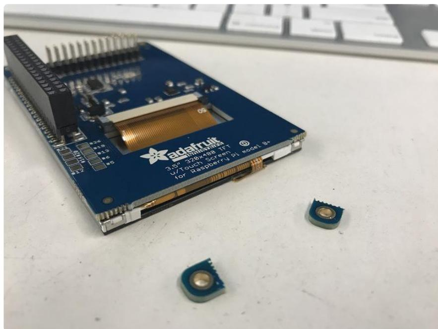
Position the PiTFT over the 2x20 GPIO connector and press downwards. Make sure the PiTFT's header is flush against the GPIO header.
