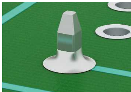
Fig. 66*: Residual ring coverage on secondary side, ideally fully wetted, min. 75%
