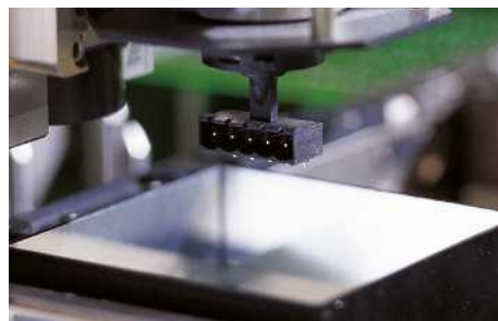
Fig. 50: Camera image capture for component measurement
