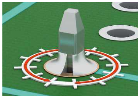
Fig. 64*: Wetting of secondary side 330° or 92%
