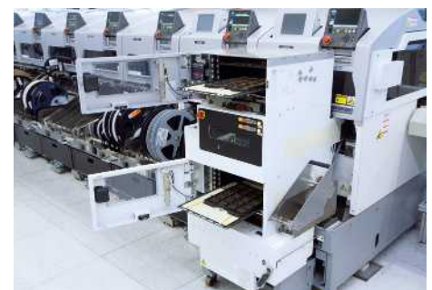
Fig. 57: Tray feeder unit (tray tower)
