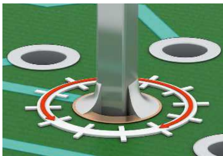
Fig. 63*: Wetting of primary side 270° or 75%
