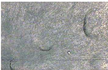
Fig. 29: Failed level – blister formation
