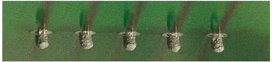
Fig. 58: Paste drops on pin tips
