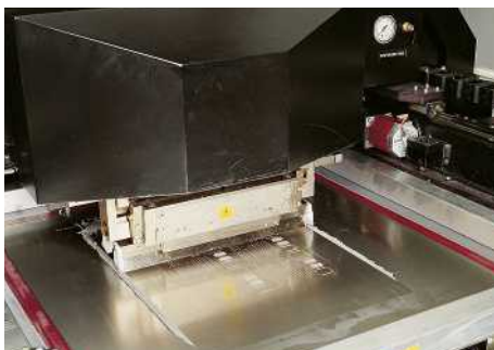
Fig. 40: Squeegee blade system for applying solder paste
