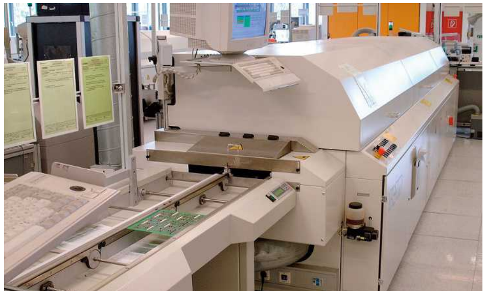
Fig. 60: Convection soldering oven
